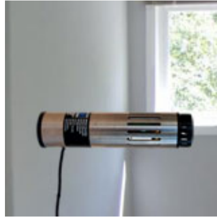
Example of a wall-mounted GrayWolf Probe
